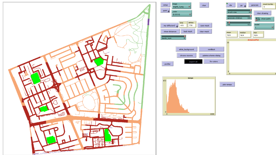
FIGURE 3. The interface of the simulation environment shows the resulting analysis on the left viewport and the different interaction widgets (buttons, plots, monitors) on the right side. The interface was designed to be expanded further with new models of pedestrian movement.
